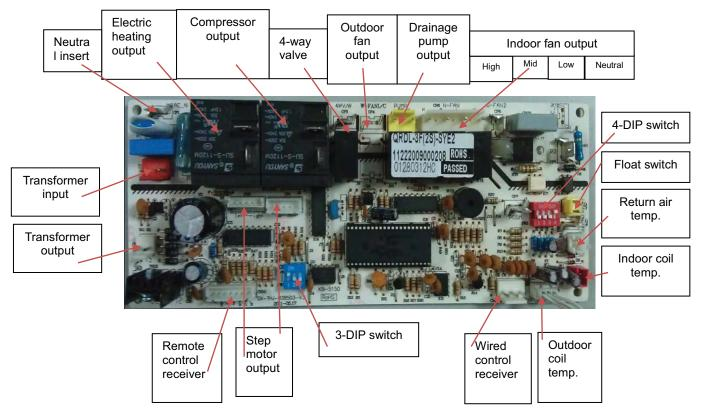
Introduction of control board QRD-SN3F(2S)-SYE1 sockets (Indoor unit) (match with the outdoor unit which the Power supply is 380V-415V, 3PH)
