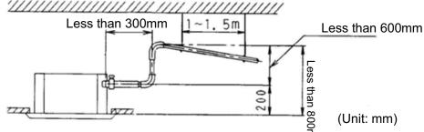
♦ When draining multiple units into a common drain line, this common drain should be installed about 100mm below each units drain outlet, as shown in the drawing.
