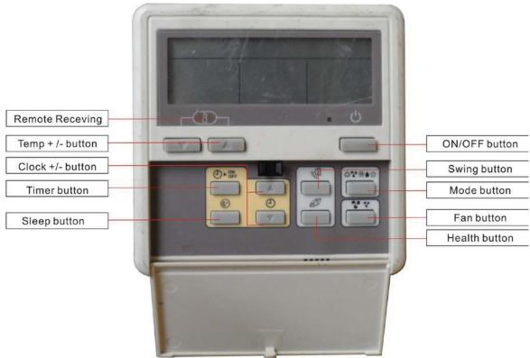
ON/OFF button: Switch the unit ON/OFF.
