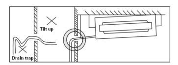
♦ When finish installation, please carry out the drainage test to ensure that the water flow through the pipeline fluently, and carefully observe the junction to ensure that there is now ater leakage at the junction. If the unit is installed in the newly built house, strongly recommend that this test taken before the ceiling installation. Even it is the heating only unit, this test is unavoidable.
